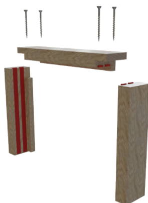
Trenched or Half Lapped Joint
