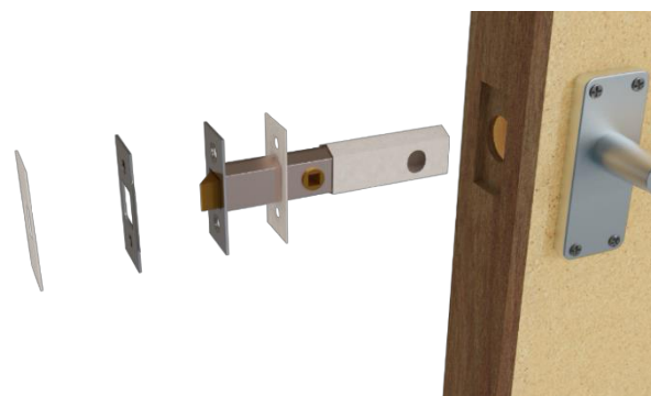
Example of lock & latch protection detail
